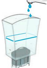
Tilt the water tank back and forth to remove air bubbles from the filter.
